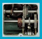
The power quill feed is electrically controlled for smooth movement and precision machining.
