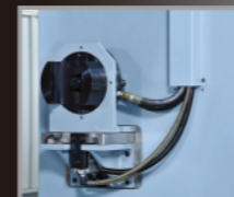
Tool changer mechanism for horizontal spindle
